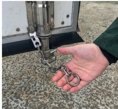
**FIGURE 5.1.25** The safety chain is placed at the bottom of the doors.
