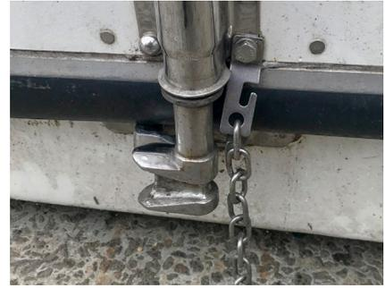
**FIGURE 5.1.23** Lock rod in secure position bottom.
