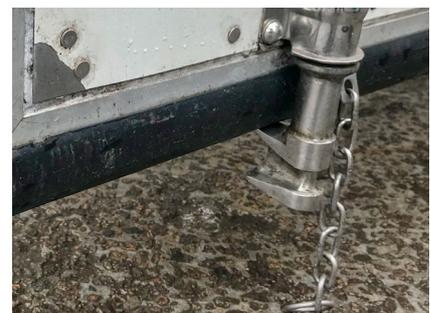
**FIGURE 5.1.20** Lock rod bottom.
