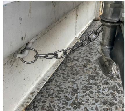
**FIGURE 5.1.26** The chain is secured to the hook on both sides of the container.
