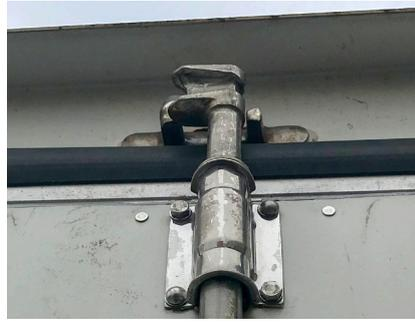
**FIGURE 5.1.22** Lock rod in secure position top.
